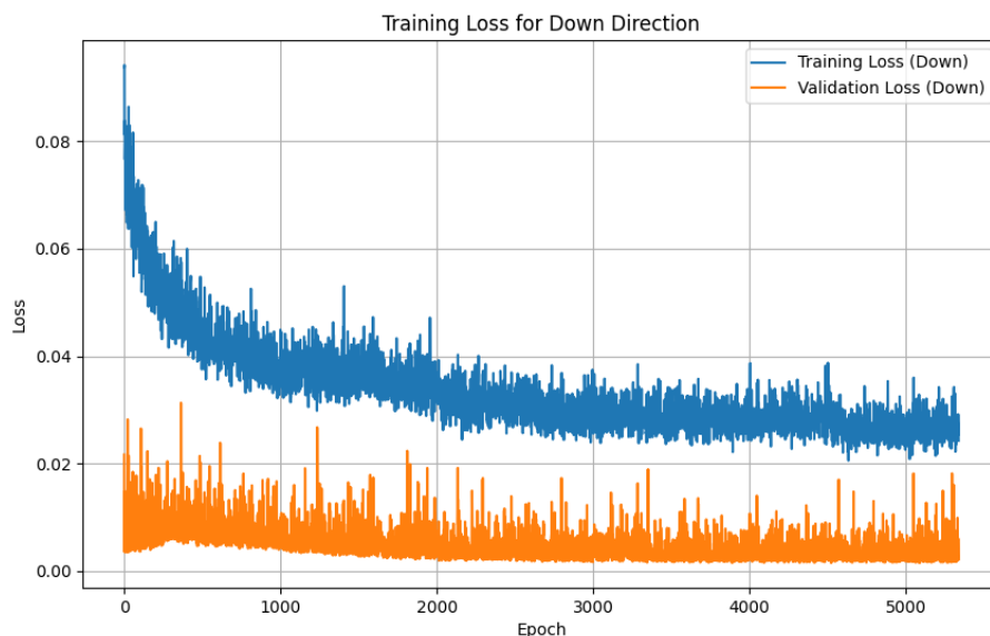
Fig. 4 Graph of the neural network loss function for predicting the unloading stage of an SMA sample
